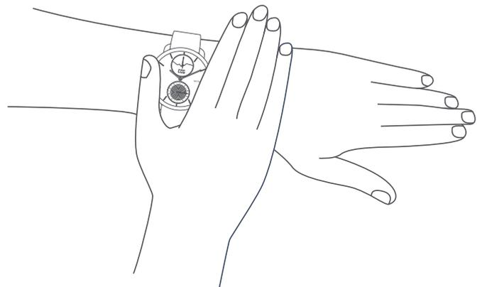
By placing his opposite hand on the watch, the user creates a closed electrical circuit with his arms and chest, allowing the measurement of a one-lead ECG.
