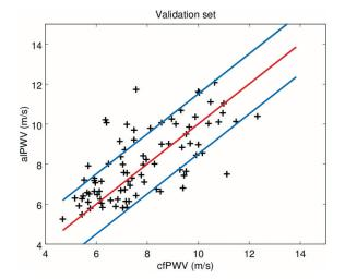
Figure 4: Estimated Body Cardio Body PWV against the reference values obtained with the Sphygmocor (correlation coefficient is r=0,72). Velocities on the red line are equal. Crosses within the blue lines are  $\leq 1.5$  m/s away from the reference value.
