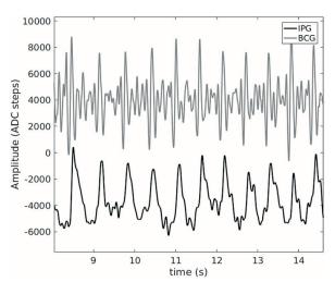
Figure 3: Ballistocardiography (BCG) and Impedance Plethysmography (IPG) signals on Body Cardio.
