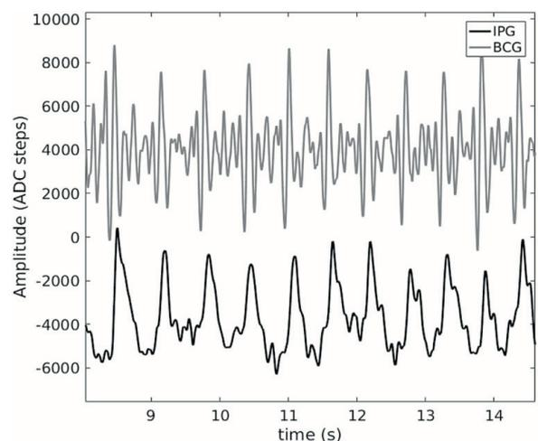
Figure 3: Ballistocardiography (BCG) and Impedance Plethysmography (IPG) signals on Body Cardio.
